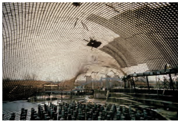
Figure 19.2 Load test where dustbins full of water were hung from the roof by wires
