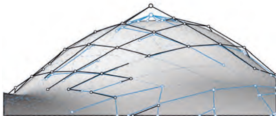
Figure 13.11 Comparison of the best-fit thrust network corresponding to the original force pattern (blue) and to the modified force pattern (black). The modified pattern clearly produces a much better fitting result
