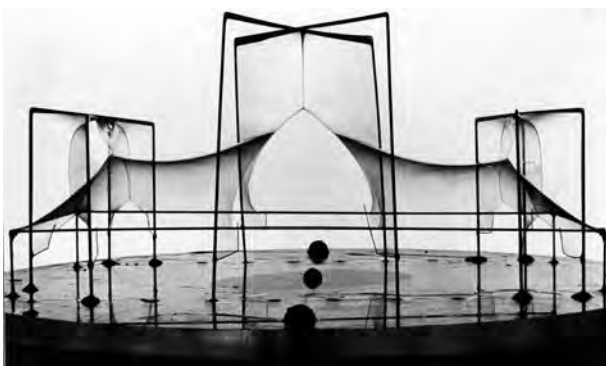
Figure 4.9 Form-finding model by Frei Otto for a tensile membrane roof, using a soap bubble approximately 1m wide. Image inverted
