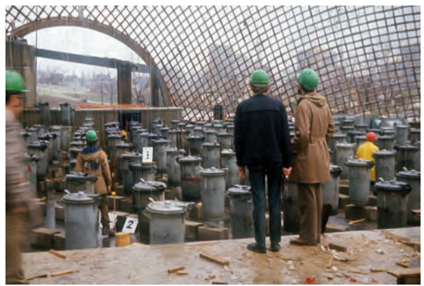
Figure 19.2 Load test where dustbins full of water were hung from the roof by wires
