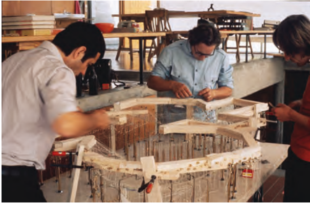
Figure 4.13 Making the 1:98.9 scale hanging-chain model to determine the precise funicular form of the Multihalle shell
