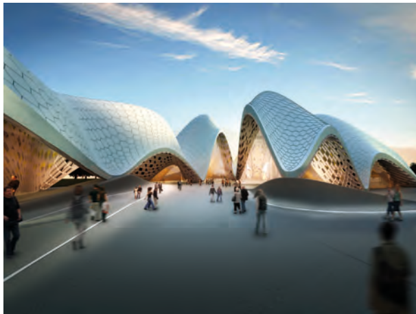
Figure 9.4: (top) Stretched cloth models result in anticlastic shells (hypothetical metro station in Bangalore), while (bottom) hanging cloth models result in synclastic shells (design entry for innovation centre in China), both designs by Zaha Hadid Architects
