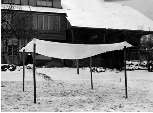
Figure 4.8 Hanging model by Heinz Isler. A wet cloth frozen during a winter night to create the form of a reinforced-concrete shell roof
