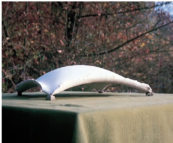
Figure 20.13 The hanging membrane, once hardened, is inverted to create a shell form in pure compression
