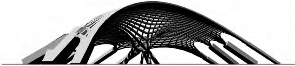
Figure 11.8 Geometric envelope based on forces present in the structure
