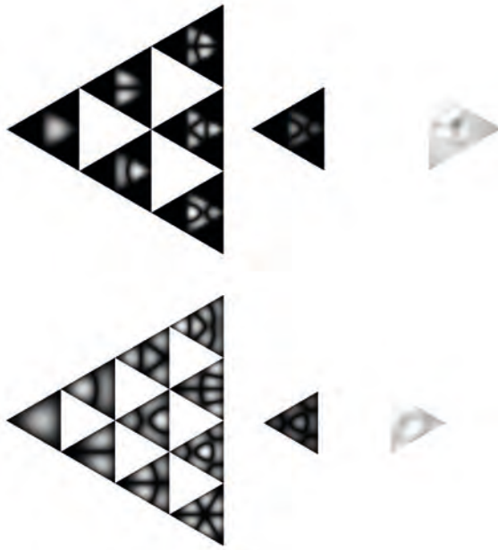
Figure 16.5 Shape optimization (top) within a subdomain (smaller triangle within larger triangle), and (bottom) full optimization with vanishing boundaries
