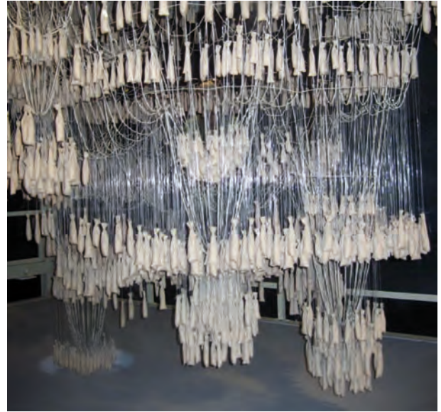
Figure 4.6 Reproduction of Gaudi's hanging model for the crypt of Colònia Güell, Barcelona
