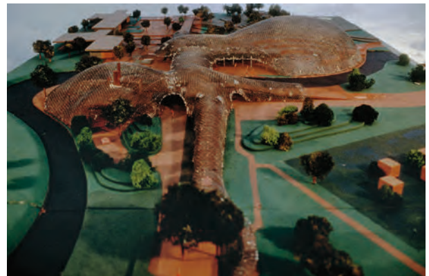
Figure 4.12 A 1:300 scale wire-mesh model of the Multihalle to establish general form
